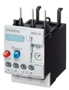
Overload relay 1.8...2.5 A For motor protection Size S0, Class 10 Contactor mounting Main circuit: screw terminal Auxiliary circuit: screw terminal Manual-Automatic-Reset !!! Phased-out product !!! Successor is SIRIUS 3RU2 Preferred successor type is >>3RU2126-1CB0<<
