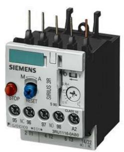
Overload relay 0.22...0.32 A For motor protection Size S00, Class 10 Contactor mounting Main circuit: screw terminal Auxiliary circuit: screw terminal Manual-Automatic-Reset !!! Phased-out product !!! Successor is SIRIUS 3RU2 Preferred successor type is >>3RU2116-0DB0<<
