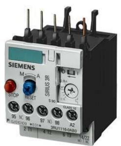
Overload relay 0.45...0.63 A For motor protection Size S00, Class 10 Contactor mounting Main circuit: screw terminal Auxiliary circuit: screw terminal Manual-Automatic-Reset !!! Phased-out product !!! Successor is SIRIUS 3RU2 Preferred successor type is >>3RU2116-0GB0<<
