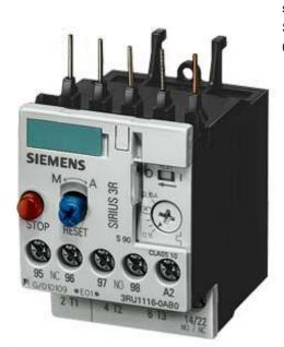
Overload relay 0.55...0.8 A For motor protection Size S00, Class 10 Contactor mounting Main circuit: screw terminal Auxiliary circuit: screw terminal Manual-Automatic-Reset !!! Phased-out product !!! Successor is SIRIUS 3RU2 Preferred successor type is >>3RU2116-0HB0<<
