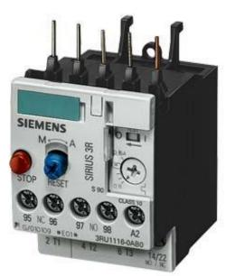
Overload relay 1.8...2.5 A For motor protection Size S00, Class 10 Contactor mounting Main circuit: screw terminal Auxiliary circuit: screw terminal Manual-Automatic-Reset !!! Phased-out product !!! Successor is SIRIUS 3RU2 Preferred successor type is >>3RU2116-1CB0<<
