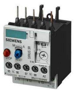
Overload relay 3.5...5 A For motor protection Size S00, Class 10 Contactor mounting Main circuit: screw terminal Auxiliary circuit: screw terminal Manual-Automatic-Reset !!! Phased-out product !!! Successor is SIRIUS 3RU2 Preferred successor type is >>3RU2116-1FB0<<
