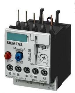
Overload relay 5.5...8 A For motor protection Size S00, Class 10 Contactor mounting Main circuit: screw terminal Auxiliary circuit: screw terminal Manual-Automatic-Reset !!! Phased-out product !!! Successor is SIRIUS 3RU2 Preferred successor type is >>3RU2116-1HB0<<
