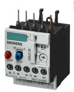
Overload relay 9...12 A For motor protection Size S00, Class 10 Contactor mounting Main circuit: screw terminal Auxiliary circuit: screw terminal Manual-Automatic-Reset !!! Phased-out product !!! Successor is SIRIUS 3RU2 Preferred successor type is >>3RU2116-1KB0<<
