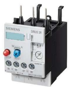
Overload relay 5.5...8 A For motor protection Size S0, Class 10 Contactor mounting Main circuit: screw terminal Auxiliary circuit: screw terminal Manual-Automatic-Reset !!! Phased-out product !!! Successor is SIRIUS 3RU2 Preferred successor type is >>3RU2126-1HB0<<
