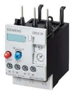
Overload relay 14...20 A For motor protection Size S0, Class 10 Contactor mounting Main circuit: screw terminal Auxiliary circuit: screw terminal Manual-Automatic-Reset !!! Phased-out product !!! Successor is SIRIUS 3RU2 Preferred successor type is >>3RU2126-4BB0<<
